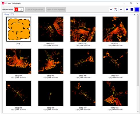
A scan thumbnail window provides the user with a clear view of all scans within a project. Scans can be viewed and aligned visually right after import.
