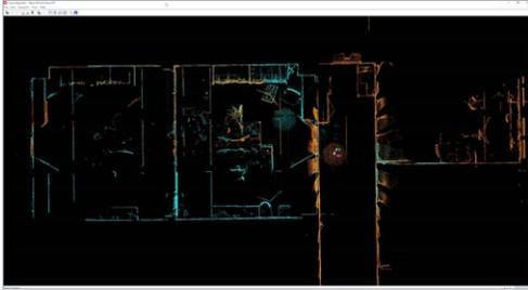
Enhanced Visual Alignment provides an automatic ortho-rectified alignment in plan view.
