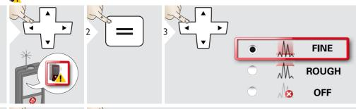
Choose the sensitivity of the levelling, which is needed for some measuring functions. FINE means, that the levelling of the device is sensitive to any small vibrations. Choose ROUGH when working in harsh construction environment with many shocks and vibrations. In this case the accuracy is decreased in correlation with the movements.
