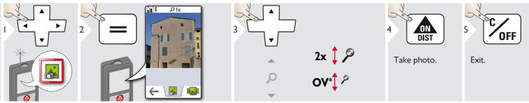
Tap on the camera icon in the middle of the bottom line to take a photo. For screenshots, press camera key for 2 sec.
