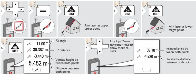
Indirect distance measuring between 2 points with additional results. Ideal for applications such as length and slope of roof, height of chimneys,...
