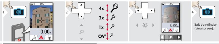
This is a great help for outdoor measuring. The integrated pointfinder (viewscreen) shows the target on the display. The device measures in the middle of the cross hair, even if the laser dot is not visible.
