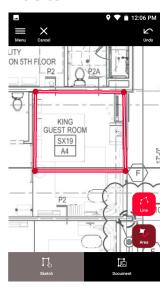
7. Select a line and press **Laser** to measure the length. Alternatively select a line and press **Enter** to add length.
