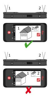
3. The intersection angle between the two lines of sight from the two cameras is key for good 3D accuracy. The angle is affected with the distance (D) to the object and the baseline length (B).
