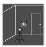
2. Fit the calibration plate into the red frame shown on screen. Use the guidelines on the screen to adjust the distance of the camera from the calibration plate (1.2 m/3.9 ft). Trigger the picture using the **Photo** button on screen.
