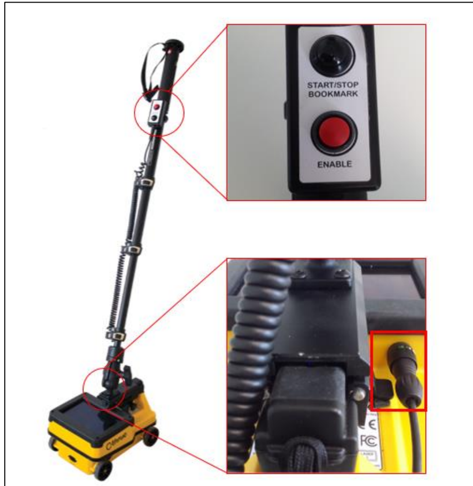
Fig. 35 – Telescopic rod final assembling
