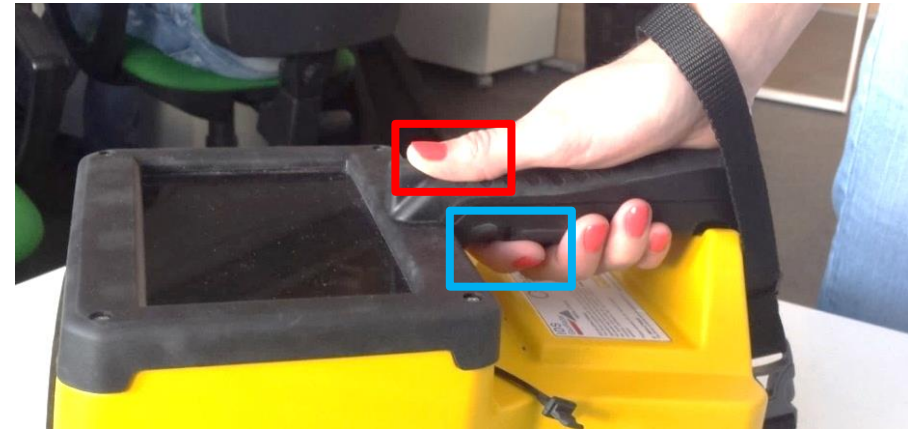
Fig. 13 – Button for start/stop acquisition and marker positioning (red square) and the additional button (blue square) for FCC regulations.
