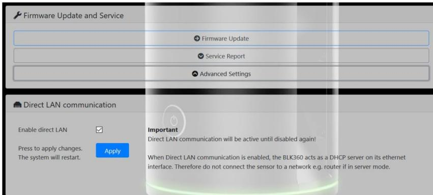
Set the tick-mark for “Enable direct LAN” and press Apply.
