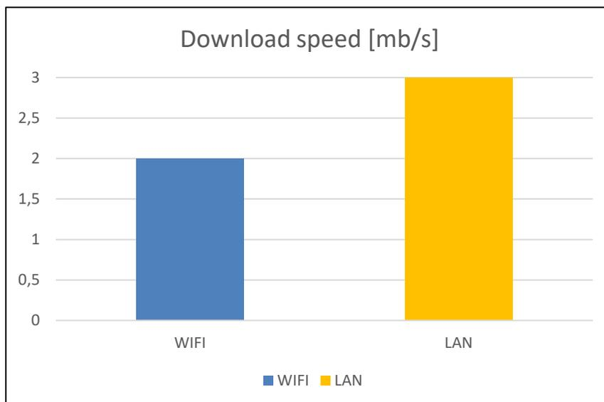
The speed of the data transfer not only depends on the used method (WiFi or LAN) but changes as well with the used computing device. For the setup using a LAN infrastructure (router) other factors will affect the speed as well. For example the general traffic within the network.
