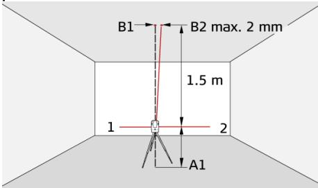
Rotate the instrument by 180° so that it points in the opposite direction 2 to direction 1. Adjust the instrument so that the laser beam hits point A1 exactly. If point B2 is no further than 2 mm away from point B1, then the instrument is within tolerance.
