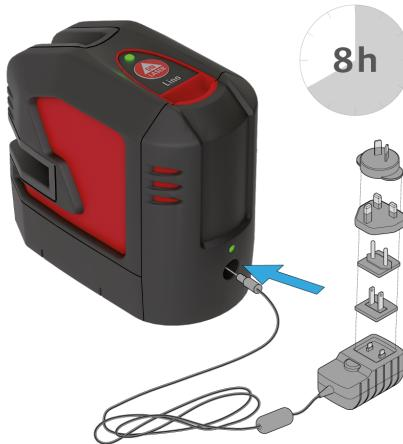
Charge the Li-Ion battery before using it for the first time. While charging, the instrument may heat up. This is normal and should not affect the instrument's lifespan or performance. At the recommended storage temperature of -20°C to +30°C (-4°F to +86°F), batteries containing a 50% to 100% charge can be stored up to 1 year. After this storage period the batteries must be recharged.
