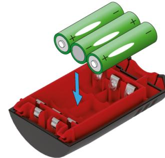
Insert Alkaline batteries in the battery-pack.
