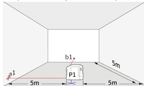
Place lock switch in "Unlocked" position (see [Levelling lock](#)). Mark a reference point (P1) approx. 5m from the walls and position the lower plumb point exactly on it. Align the cross hair to the left wall and mark the intersection point (a1) approx. on the same height like P1 to the wall. Shortly after mark the right-hand perpendicular beam (b1) on the front wall.
