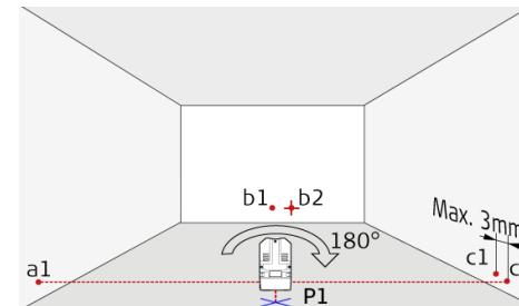
Afterwards turn the device exactly 180° around the plumb point P1 and position the right-hand perpendicular beam to the existing reference point a1. Make sure that the upper plumb point is still exactly on the reference P1. Then mark the left-hand beam to the right wall and mark it with c2. Finally measure the difference between the former reference point c1 and the new point c2. The deviation may be max. 3mm between these two points.
