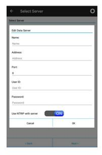
Enter a name for the data server, then the address, port and user credentials. In most cases, make sure *Use NTRIP with server* should be turned on. Tap on **OK**, then tap **Next >**.
