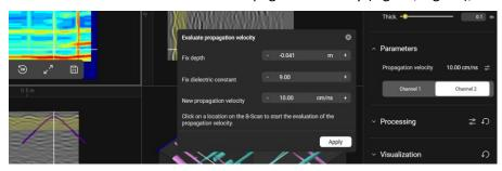
Fig. 29 Hyperbola fitting for Velocity Adjustment
